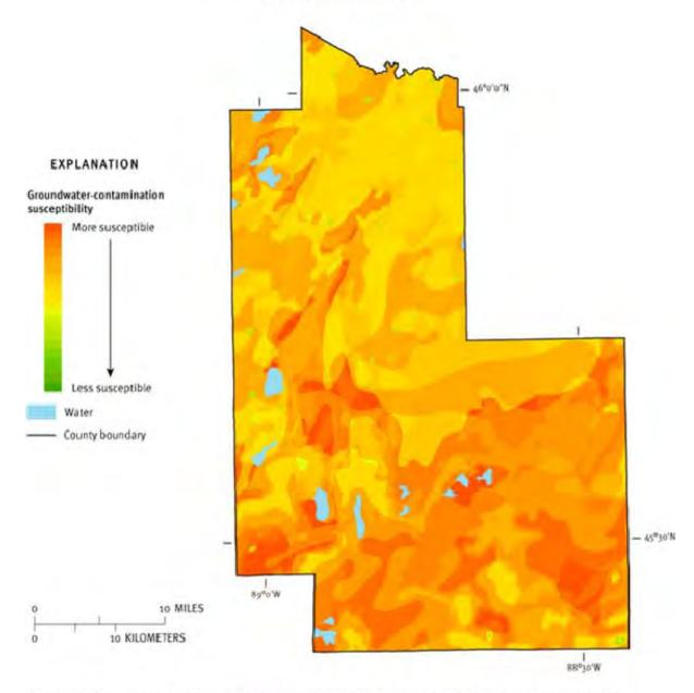
This groundwater-contamination susceptibility map is a composite of five resource characteristic maps, each of which was derived from generalized statewide information at small scales, and cannot be used for any site-specific purposes.
