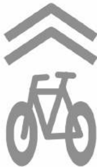
Example of "Sharrow" Pavement Marking
