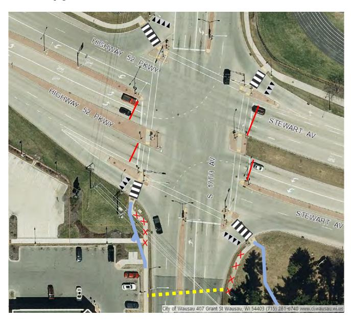
Granite or limestone boulders that you can sit on. These boulders block bicyclists from riding directly into the road without looking in the direction of traffic; thus the 90-degree bend in the sidewalk.
