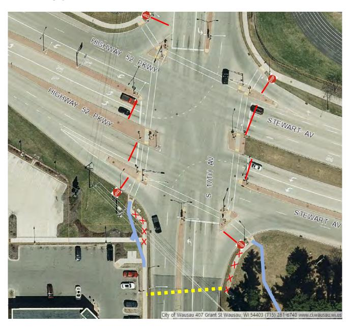
Granite or limestone boulders that you can sit on. These boulders block bicyclists from riding directly into the road without looking in the direction of traffic; thus the 90-degree bend in the sidewalk.
