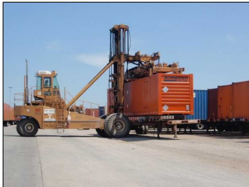
Figure 7 Top Pick Lifting a Domestic Container (Photo Dr. Richard D. Stewart)
